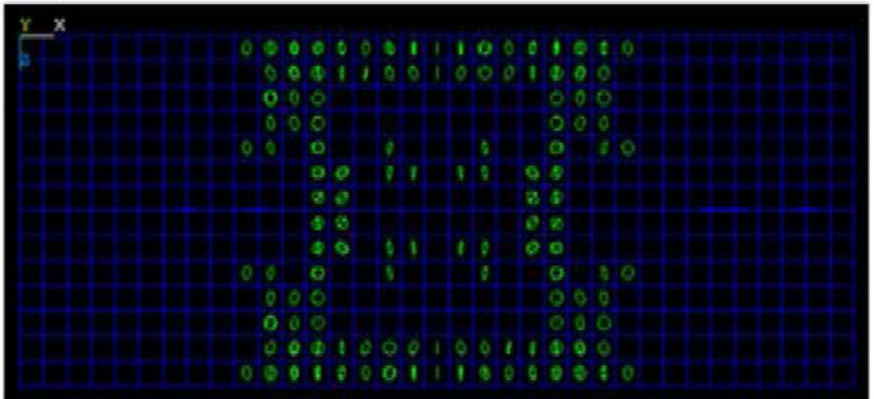
Fig. 13. NLFE Cracks Patterns; a) slabs Reinforced by steel bars; b) slabs reinforced by BFRP bars.
