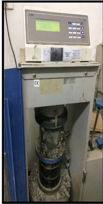
Fig. 3. concrete cubes and crushing machine of examined mix.
